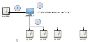
(1) Connection between the "Master" Recorder and the PC Software
